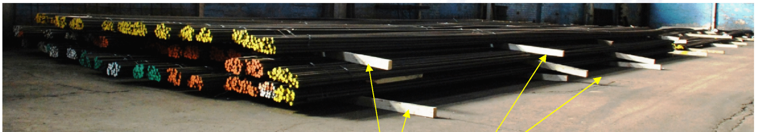
Supports – max 3 meters apart
